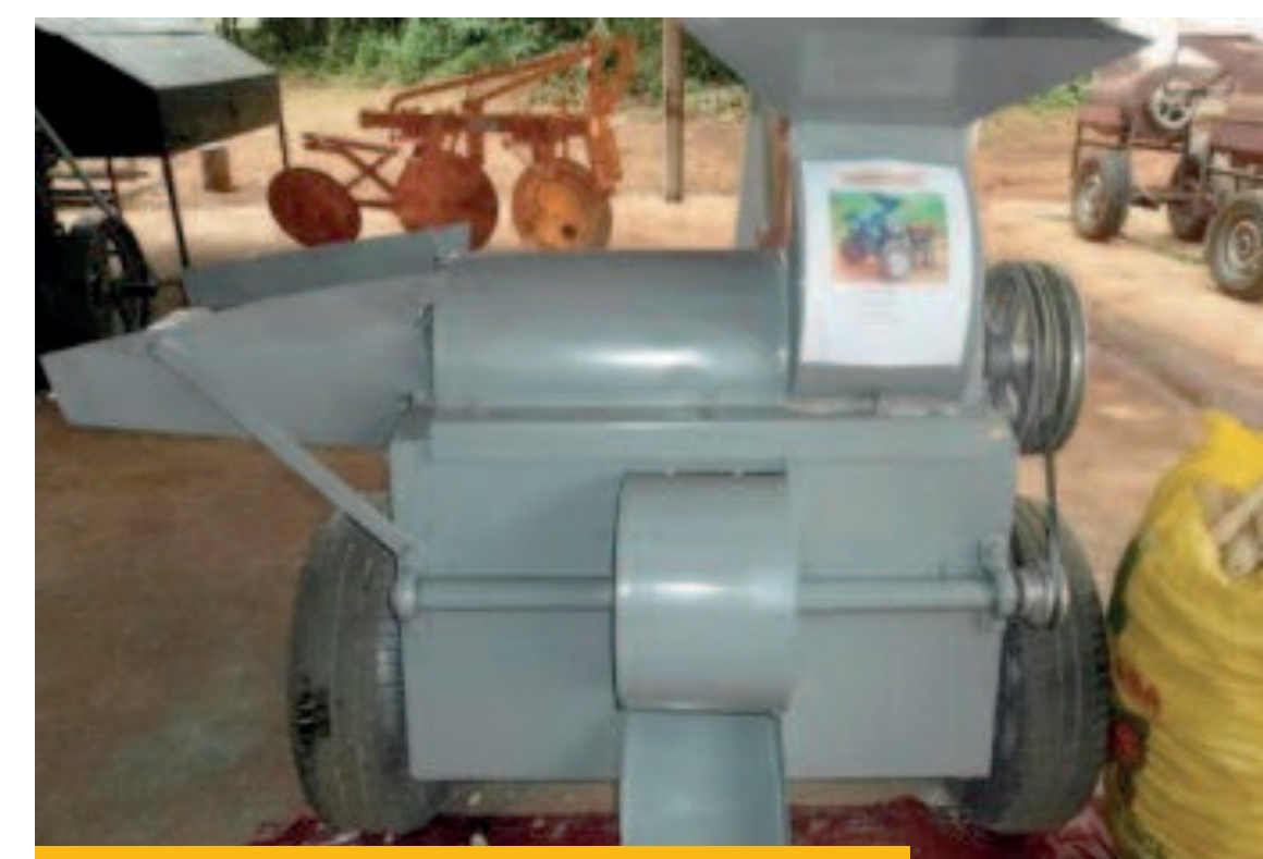
Figure 2: Aziza maize sheller and winnower
